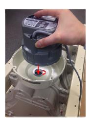
17. Put the speaker cable through the cable hole of the Driver Cover (D), and fix the clamp.
