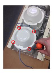
18. If you purchased "HA-450H", adjust the transformer's impedance to meet your system design. (The factory setting is 50W@70V.)
