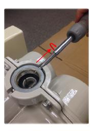
11. Tighten the side screw to fix the Adapter.
