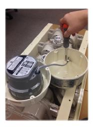
19. Fix four screws on the Driver Cover.
