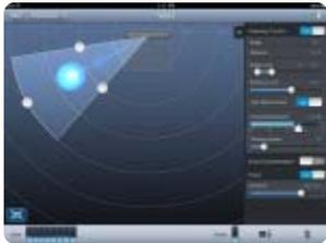
Speaking of software, the free AM-1 control app offers system config parameters, realtime visual monitoring of sound source location and gain, meters for the eight individual capsules and the output, control of the tracking range (angle and distance), tracking sensitivity and speed, gain compensation, distance adjustment threshold and more.
