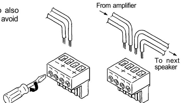
2-4. Attach two impedance selector sockets to the connector to select the desired impedance. Preset to 830 Ω (12 W for 100 V line and 6 W for 70 V line).
