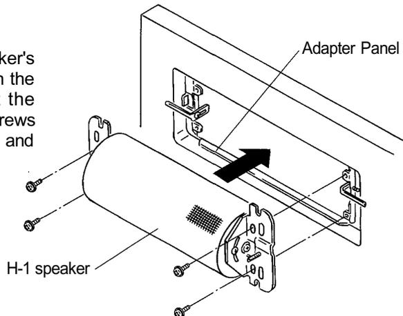
3-2. Loosen the angle adjustment screws. After adjusting the angle, retighten the screws.
