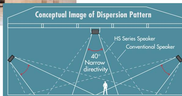
In locations with high ceilings, wide-directivity speakers cause the audio reaching the listeners to lose clarity due to overlapping of attenuated sounds.
