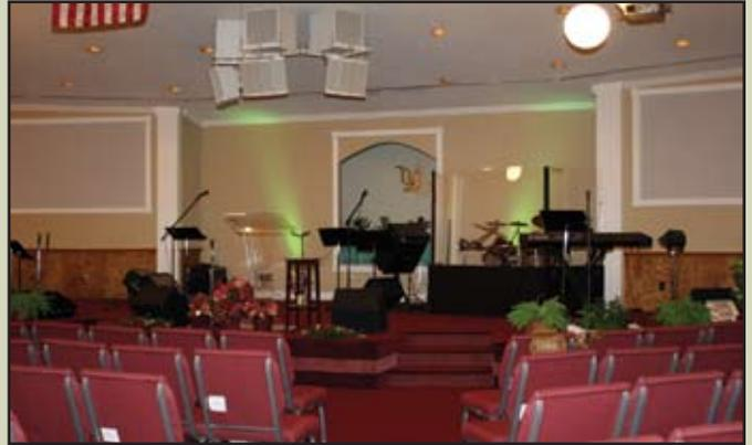
centrally located cluster is designed to provide 100-degree vertical x 150-degree horizontal dispersion pattern.
