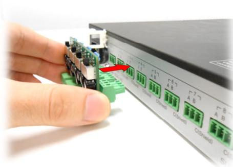
**Note:** When mounting on ports 1 through 4, please lift up the cable clamp as shown below.
