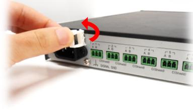
**Step3.** Wire the 3pin removable terminal plug which is supplied with N-8000/8010RS, and insert it into the terminal block on the Q-N8000LC. The other end of this wire connects to the corresponding device.
