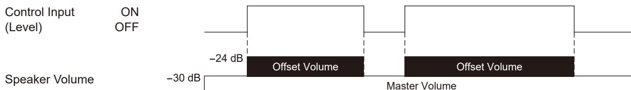
Offset Volume is applied while the Level signal is being received. Offset Volume is also applied to the audio of the ongoing broadcast in real time. This enables the audio volume control to be linked to the control input.
